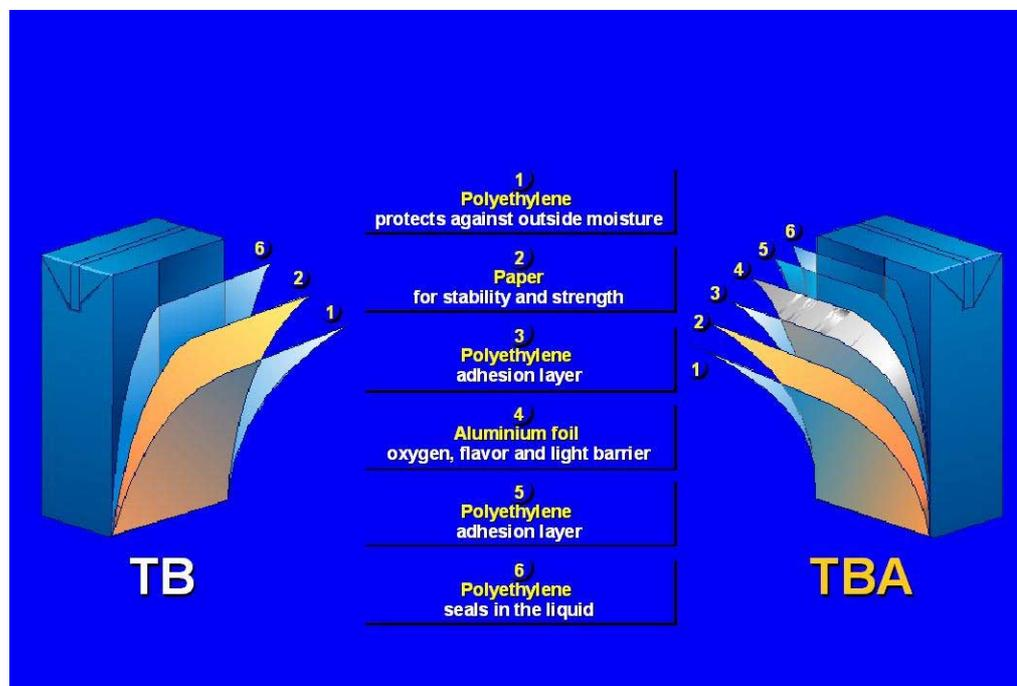
Figure 1: Laminate structure of the TB and TBA packaging materials.
