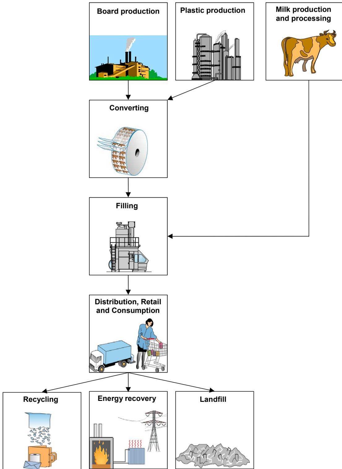
Figure 3: Main process steps of the TB/milk system. Transport steps are not displayed.
