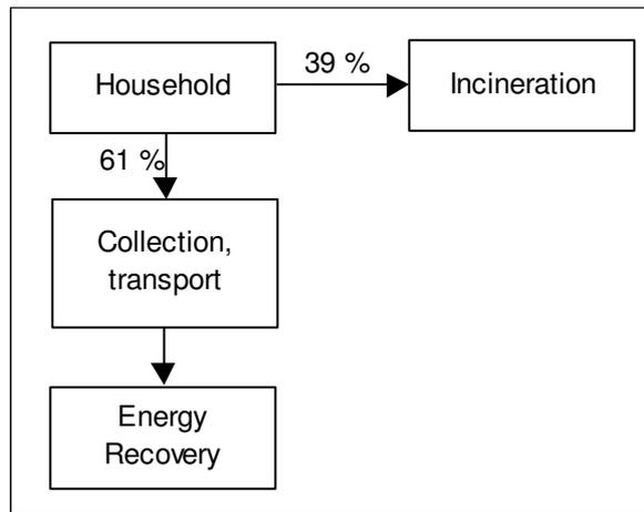
**Figure 5:** Energy 61%': source sorting with 61% collection rate and energy recovery in Denmark.
