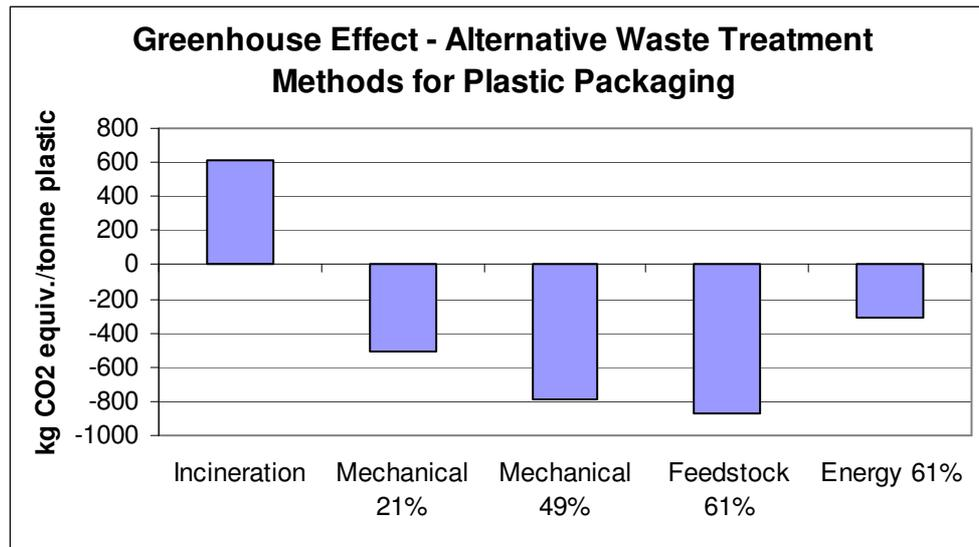
**Figure 7:** Contribution to the greenhouse effect potential for the different plastic packaging waste treatment alternatives.
