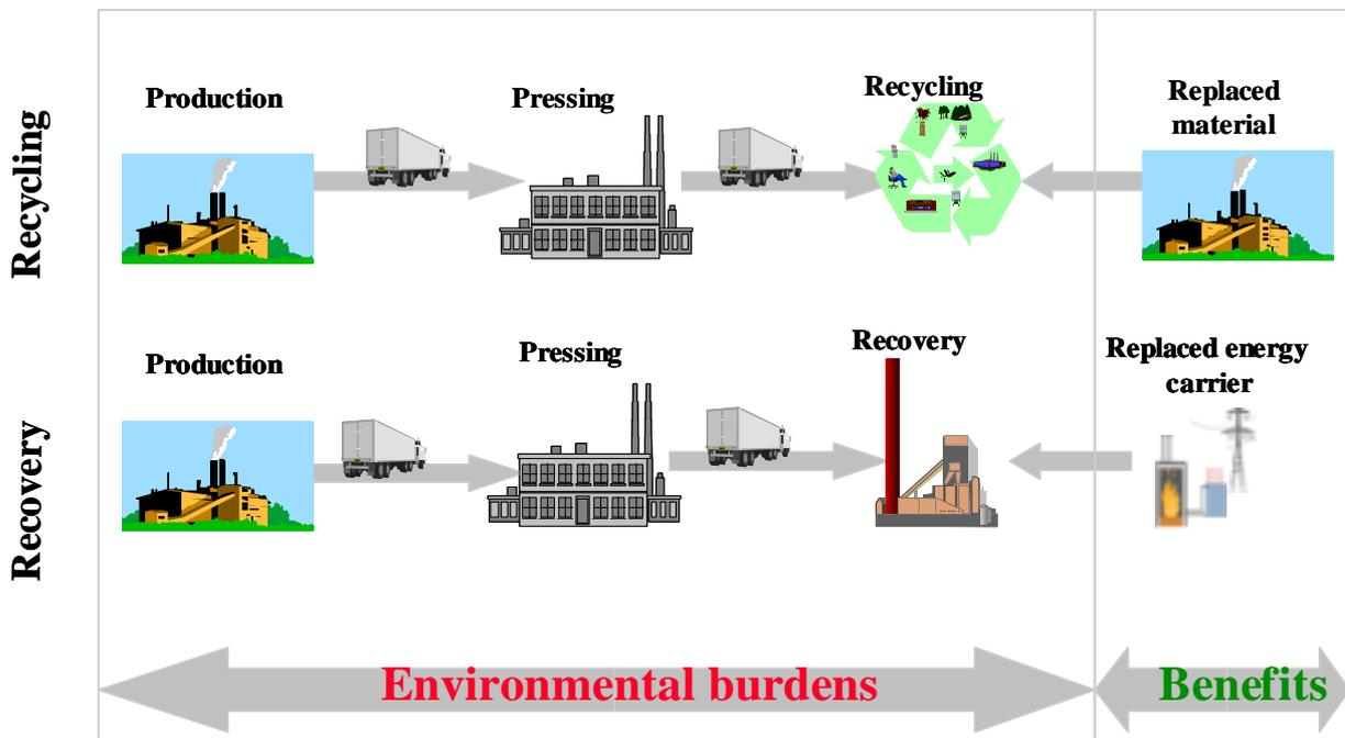
**Figure 3.1:** Flow diagram for calculation of the environmental benefits and costs of waste treatment for EPS fish containers.
