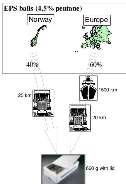
**Figure 3.2:** Flow diagram for production locations and associated transport of polystyrene balls for production of EPS fish containers.
