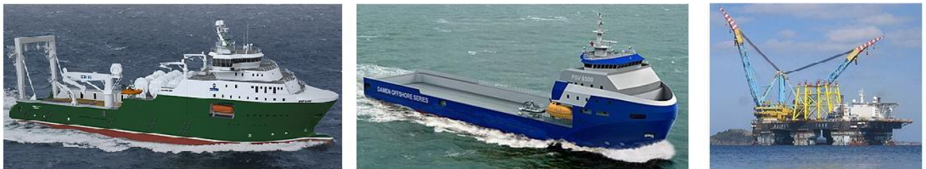
Figure A: Three AHTS', one PSV and one offshore crane is needed per installed wind turbine (Photo: Hayvord Group, NauticExpo, and Wikipedia)
